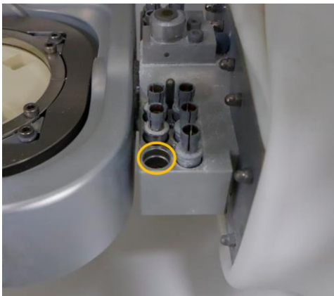
Clean the inside of pocket and spread the inside of pocket and spread the glass, such as WD40.
